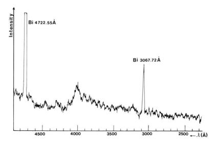
Fig. 1. Part of fluorescence spectrum of bismuth upon pure visible excitation (532 nm).
